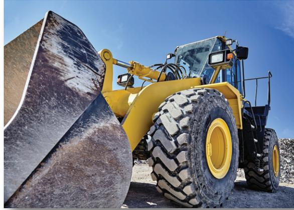
Off-Highway Research classifies wheeled loaders in two distinct types. Compact wheeled loaders from 30-80 horsepower and larger machines of 80 horsepower or more.
